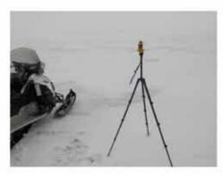
Weather monitoring using the Kestrel 5500 Weather Meter
